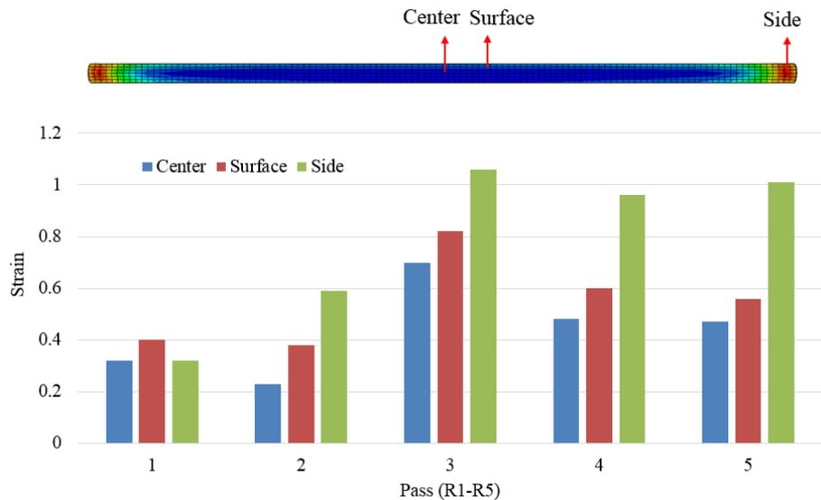
Figure 10. Comparison of plastic strain at each pass
