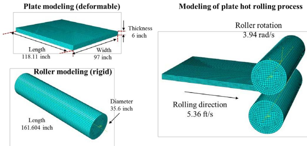
Figure 2. Schematic of the plate hot rolling
