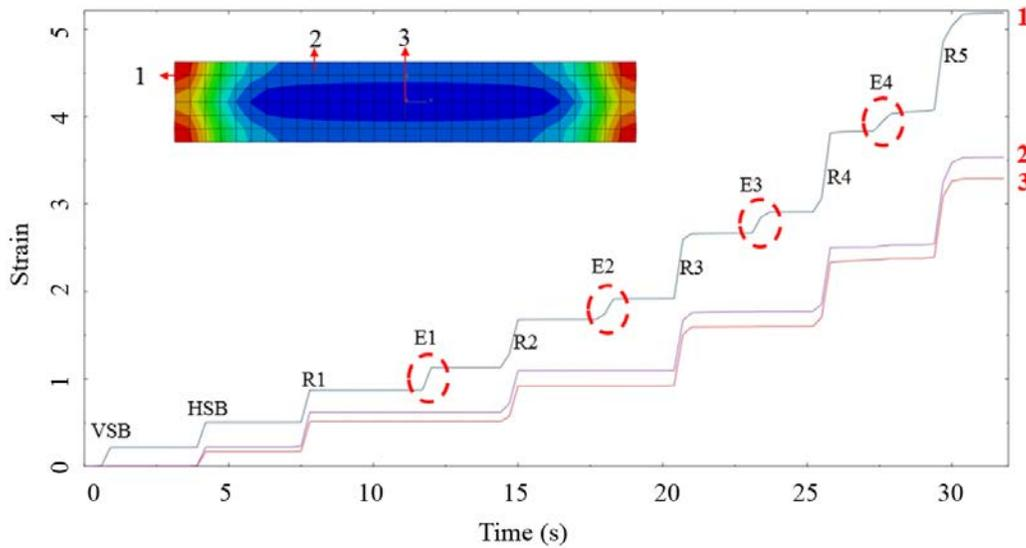
Figure 8. Accumulated plastic strain during strip hot rolling
