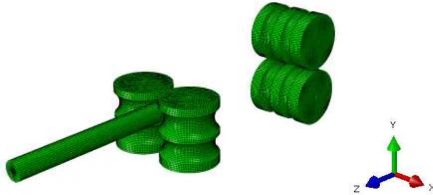
Figure 2. Modeling of round bar hot rolling process
