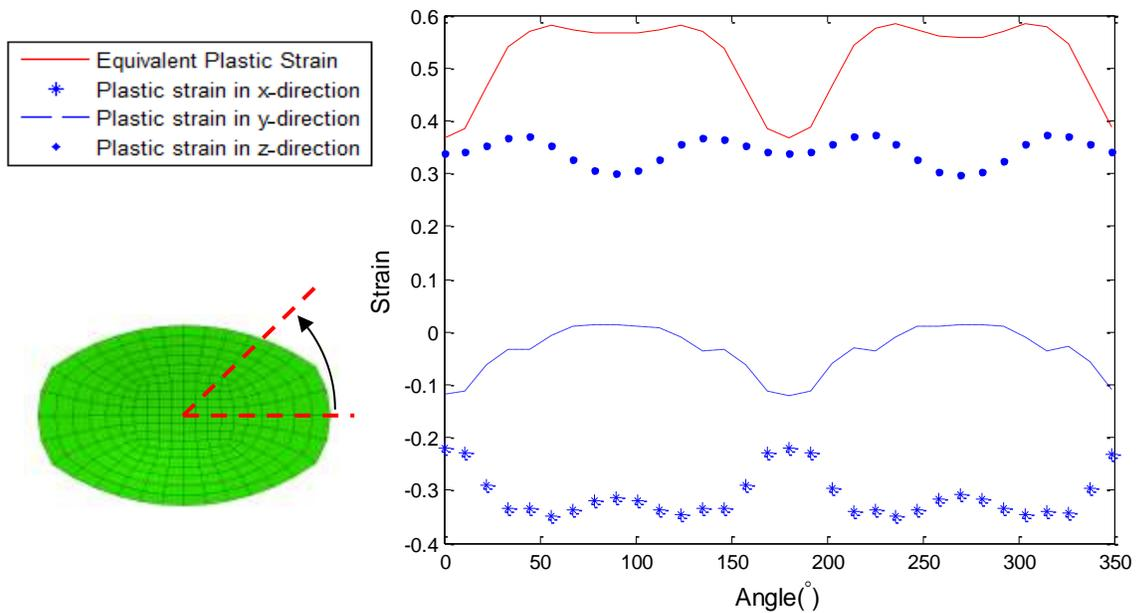
Figure 5. Plastic strain distributions along surface after stand 1
