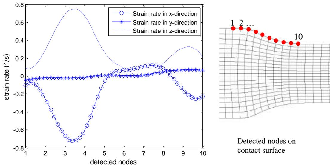
Figure 9. Strain rate distribution on contact region of stand 1
