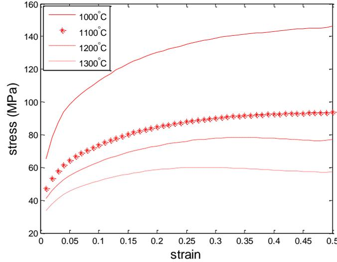
Figure 1. Stress-strain curves of 15V38 under strain rate 1 s<sup>-1</sup>
