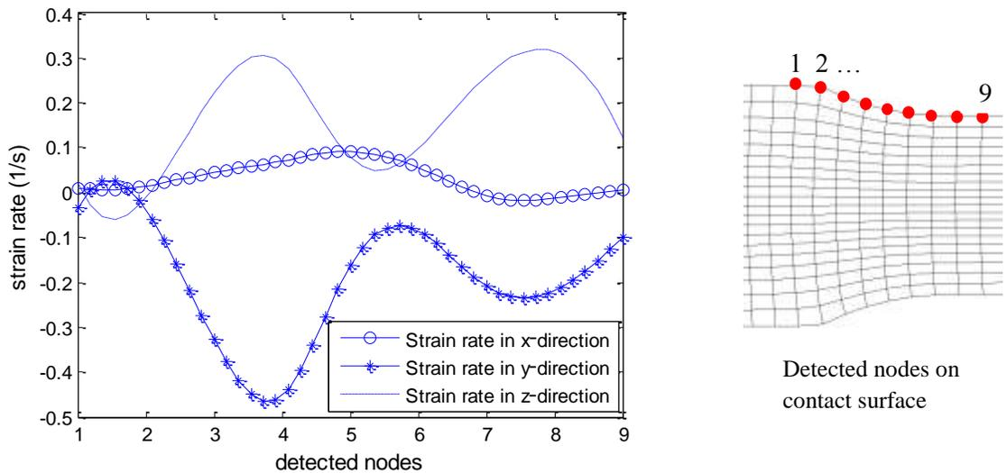
Figure 10. Strain rate distribution on contact region of stand 2
