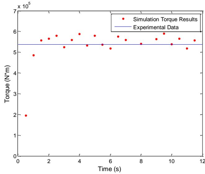
Figure 3. Stand 1 torque comparison of experimentally measured and simulated results
