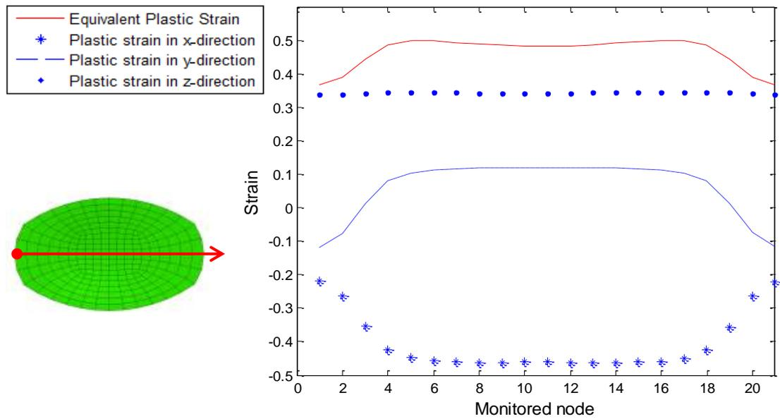
Figure 6. Plastic strain distribution of horizontal nodes after stand 1
