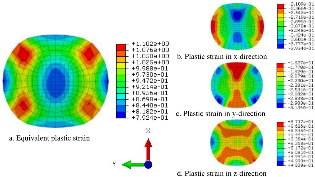
Figure 7. Equivalent plastic strain distribution of bar after stand 2
