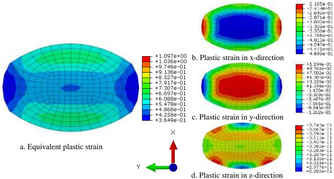
Figure 4. Plastic strain distributions of 15V38 steel bar after stand 1
