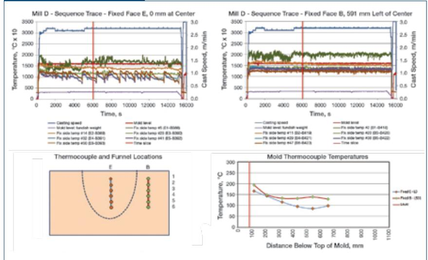
Temperature trends inside and outside of the mold funnel area over 4.5 hours of operation with flux D2 at Company D casting a 0.25 carbon steel.
