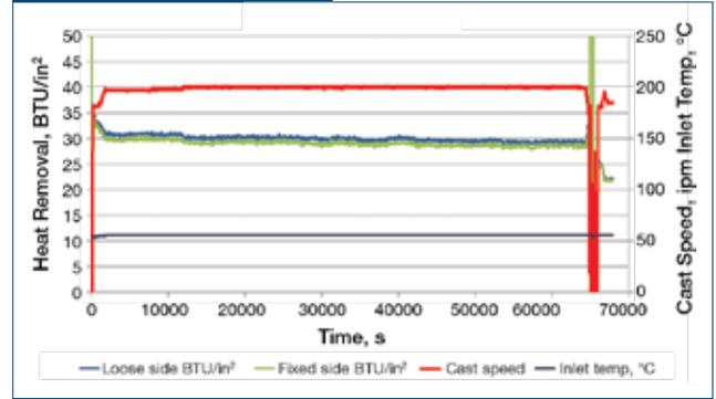
Mold heat removal for 1026 steel cast with Flux G2 at Company G.
