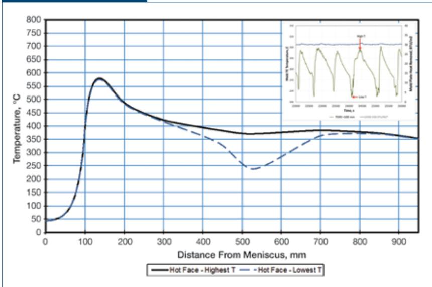
Predicted mold plate surface temperature profiles for high- and low temperature conditions shown in Fig. 12.
