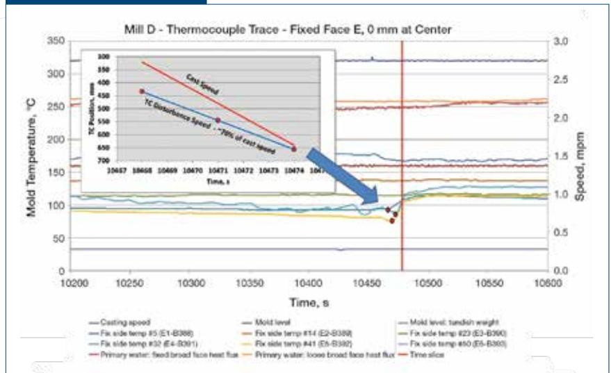
Rate of propagation of thermal disturbance past successive thermocouples in funnel area at Company D compared to casting speed.
