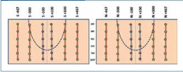
Thermocouple locations in funnel mold at Company G. Numbers shown are in mm from center or top of mold.
