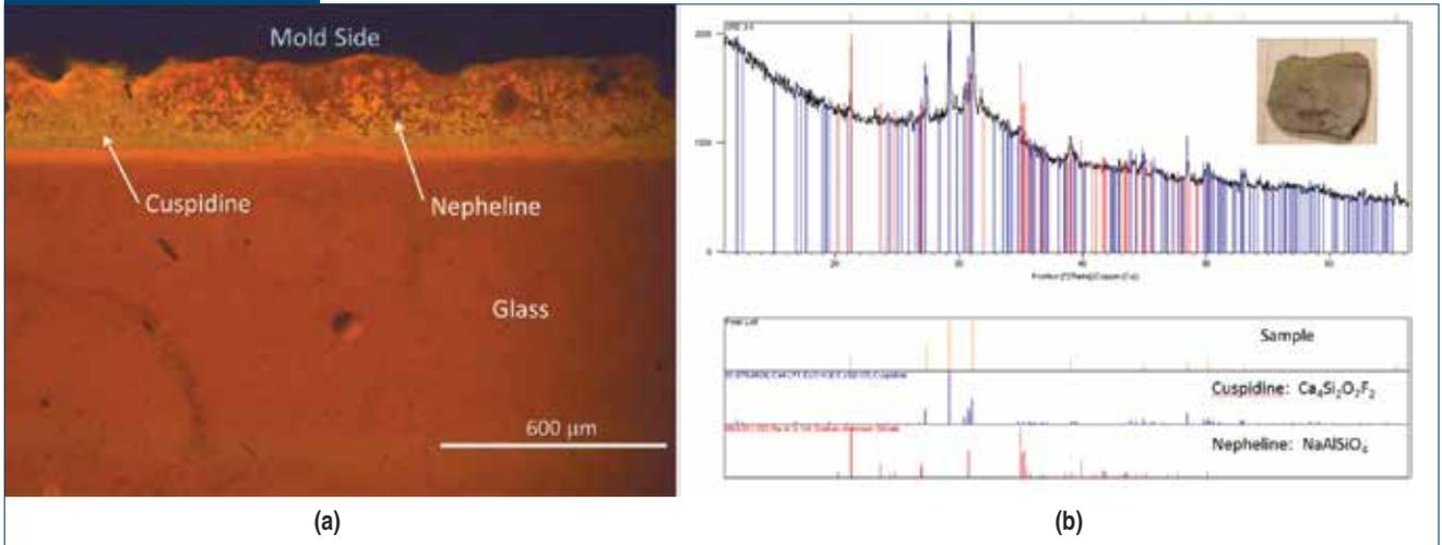
CL image of crystalline layer in G2 flux film sample showing evidence of Cuspidine and Nepheline phases (a).<sup>11</sup> Phases confirmed by x-ray diffraction analysis (b).
