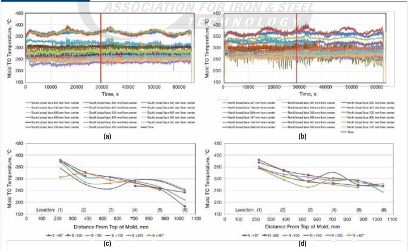
Thermocouple mold broad face temperatures for 1026 with Flux G2 at Company G (a and b) and snapshot of temperature profile on north and south broad face plates at 31,000 seconds (c and d) at red vertical line in upper figures.
