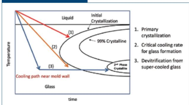
Typical continuous cooling transformation diagram showing alternate paths for crystallization.
