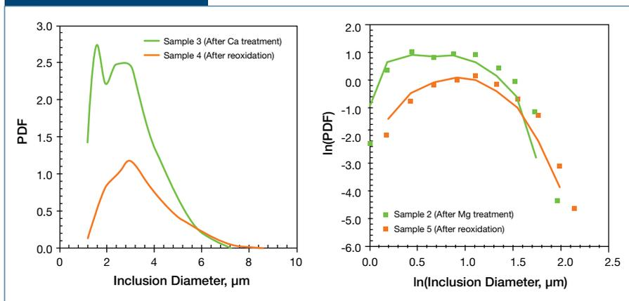
Size distribution of calcium aluminate inclusions in heat 3. Quadratic size distribution of calcium aluminate inclusions observed before and after reoxidation suggests that these inclusions were still reacting when the liquid steel was sampled. This suggests more time is required between sampling.
