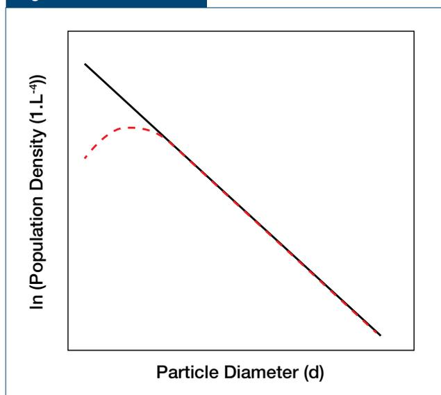
Particle distributions and the mechanism of formation. Mechanism proposed by Marsh. Distribution starts as linear and transforms to quadratic shape due to Ostwald ripening.
