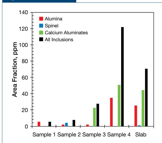
Area fraction of inclusions in samples of heat 1. A higher area fraction of spinel inclusions was observed in the slab sample (position 3) due to higher magnesium at the surface of the liquid steel.
