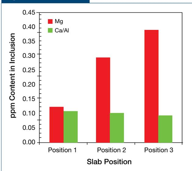
Magnesium and Ca/Al ratio of inclusions at the different slab positions. Position 3 represents inclusions at the top of the liquid steel and has the highest magnesium content in inclusions due to faster removal of magnesium vapor.
