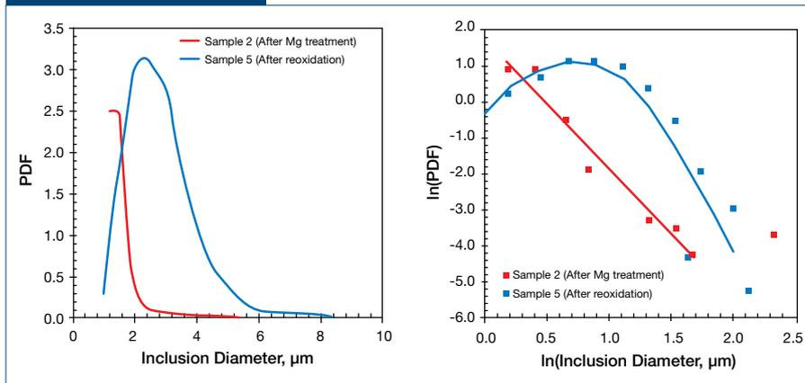
Size distribution of spinel inclusions in heat 3. Linear size distribution of spinel inclusions observed before reoxidation suggests that the inclusions were in equilibrium with the steel. After reoxidation, a quadratic distribution is observed and the spinel inclusions are larger in size.
