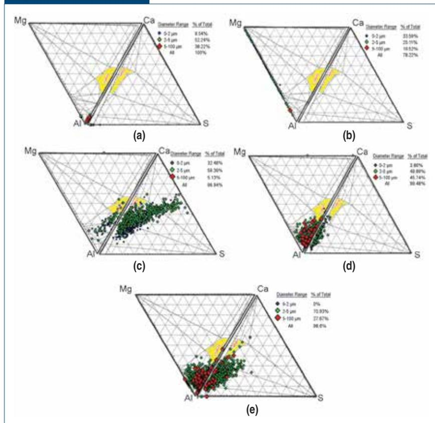
Inclusion evolution for heat 1: after deoxidation (S1) (a), after addition of magnesium (S2) (b), after calcium treatment (S3) (c), after reoxidation (S4) (d) and slab sample (e).
