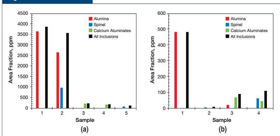
Area fraction of inclusions in heat 2 (a) and heat 3 (b). The area fraction of the inclusions in heat 2 are about seven times more than that observed in heat 3 due to the higher initial oxygen content (O) at start of the experiment in heat 2.
