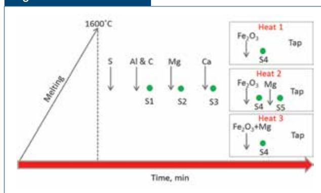
Schematic of the three heats and the respective alloying and sampling schedule.
