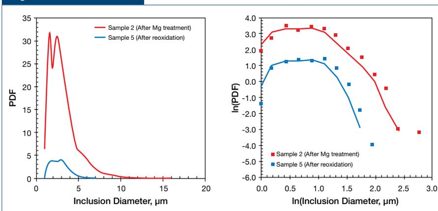
Size distribution of spinel inclusions in heat 2. Quadratic size distribution of spinel inclusions observed before reoxidation suggests that more time is required between sampling.
