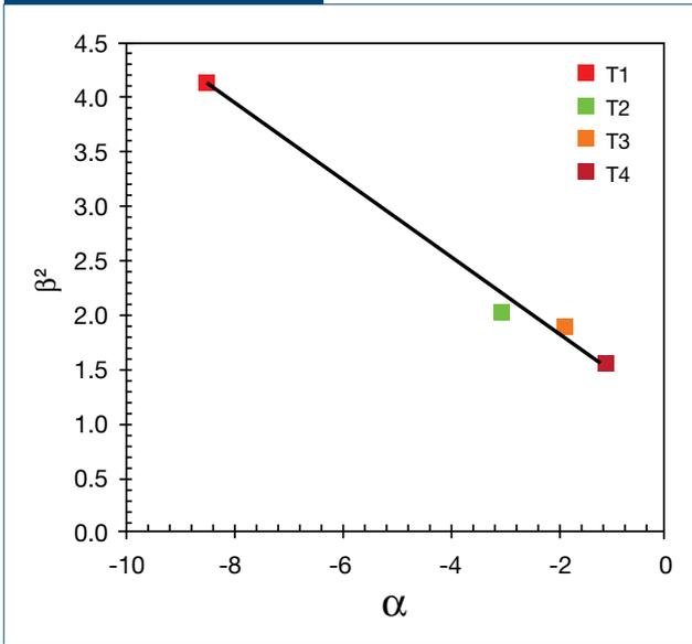
Plot of  $\beta^2$  and  $\alpha$  for samples taken from the tundish. The observed negative slope suggests the shape change resulted from Ostwald ripening.
