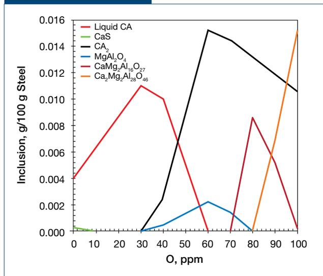
Thermodynamic simulation of the inclusion evolution in reoxidized calcium-treated steel. Newly formed spinel inclusions are observed in steel reoxidized with 30 ppm oxygen.
