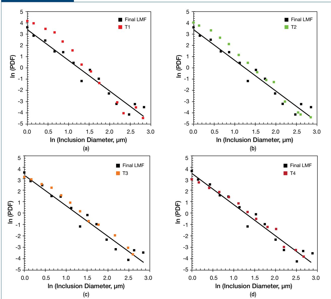
Size distribution of oxide inclusions observed in tundish samples taken from a start-up heat: positions 1 (a), 2 (b), 3 (c) and 4 (d).
