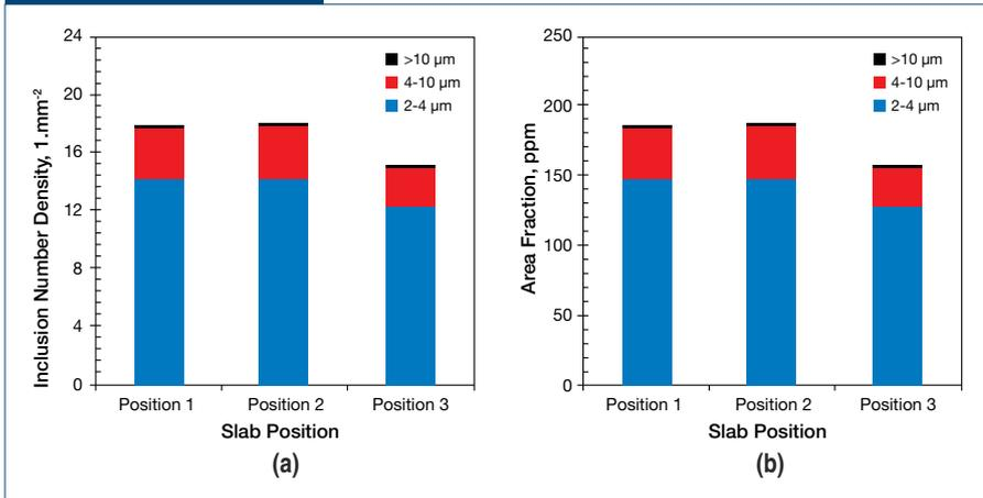
Number density and area fraction of inclusions at different positions in the slab.
