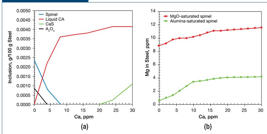
Thermodynamic simulation of spinel modification by calcium using Factsage v6.4. Target liquid inclusions form between 10 to 20 ppm Ca. Dissolved magnesium also increases during the process.
