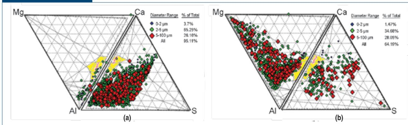
Composition of inclusions in heat 3: after calcium treatment (S3) (a) and after co-addition of magnesium and  $Fe_2O_3$  (S4) (b).
