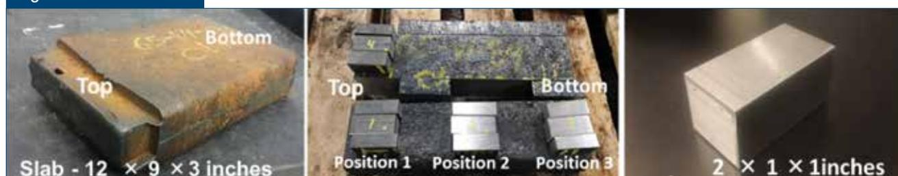
Slab sample positions sectioned for inclusion analysis. Position 1 represents the top of the slab after hot top had been sectioned out. Position 3 is the bottom of the slab and represents inclusions at the top of the crucible.
