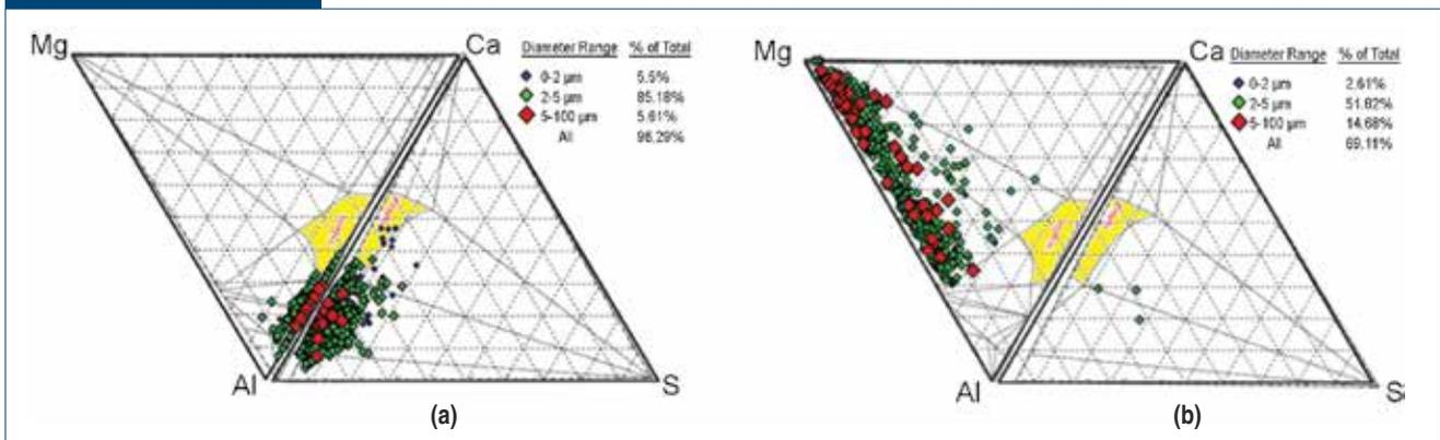
Composition of inclusions in heat 2: after calcium treatment (S3) (a) and after reoxidation and addition of magnesium (S5) (b).
