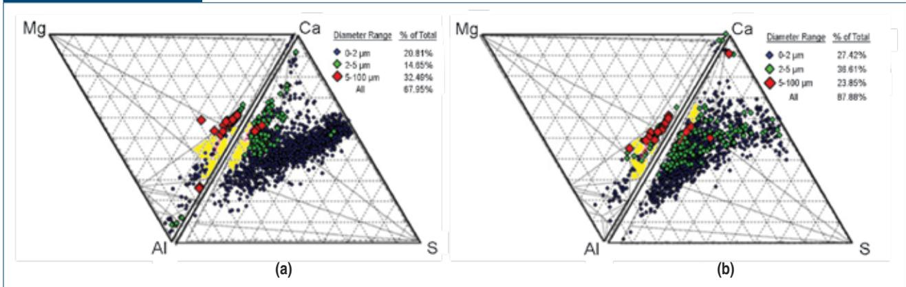
Inclusion composition at final LMF (after Ca treatment) (a) and tundish (duration T1) (b). Presence of fine alumina inclusions in the tundish is evidence of reoxidation during transfer.
