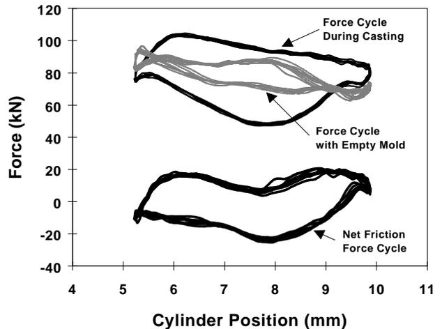
Fig. 15. Force vs. cylinder position for empty mold and during casting, and net friction force determined by difference.
