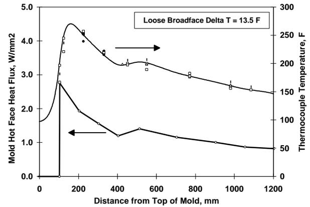
Fig. 13. Mold hot face heat flux profile for 409 at 60 ipm determined by fitting mold thermal model results to measured thermocouple temperatures and mold water heat extraction.
