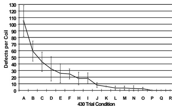
Fig. 23. Reduction of caster fold defects on 430 stainless at Mansfield by trial condition.
