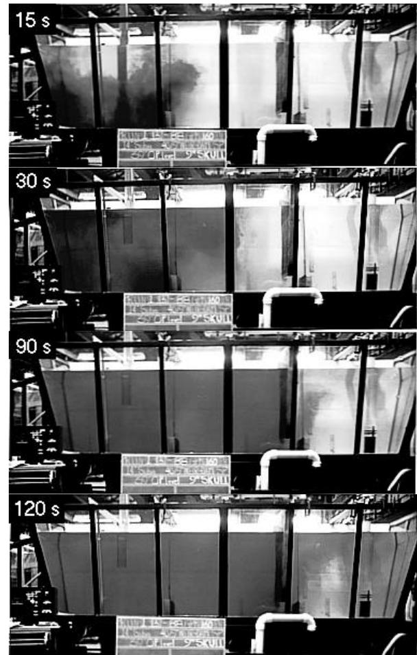
Fig. 2. Visible dye injection sequence in tundish water model at 160 TPH.
