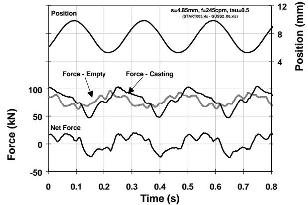
Fig. 14. Net friction force extracted from oscillator cylinder hydraulic pressure measurements.
