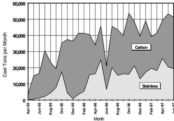
Fig. 24. Carbon and stainless production at Mansfield Operations.
