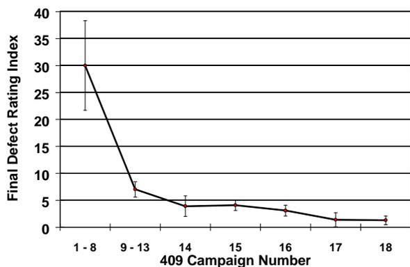
Fig. 21. Progression of hot band surface quality improvements on 409 stainless at Mansfield.
