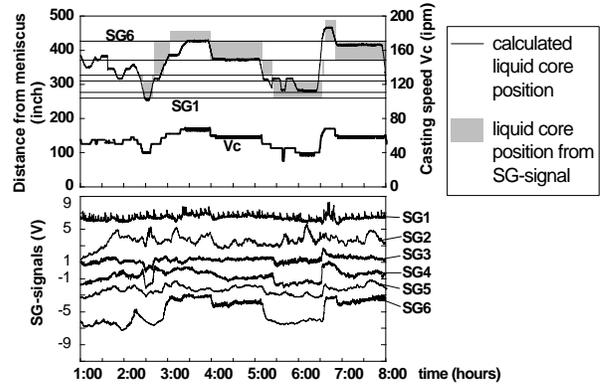
Fig. 20. Comparison of measured and predicted liquid core position for low carbon steel.
