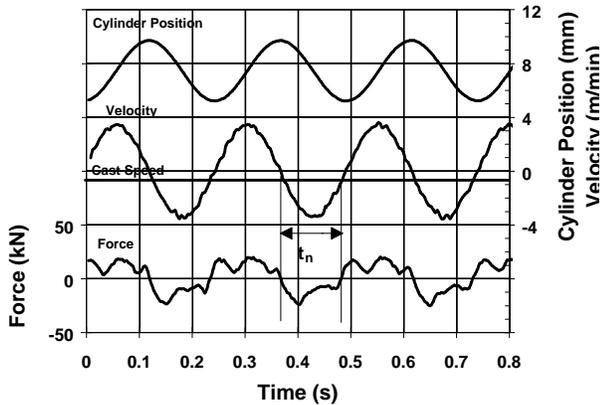
Fig. 16. Net strand friction force over several oscillation cycles.
