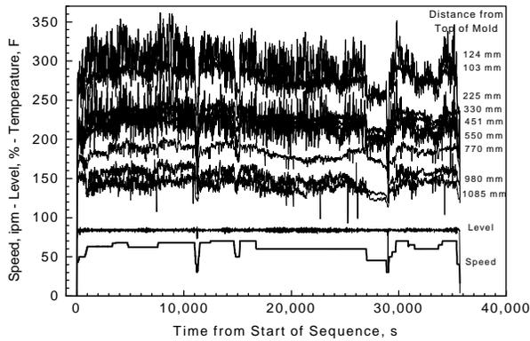
Fig. 11. Typical mold thermocouple temperatures from an 8 heat sequence of 409 stainless. Fixed broadface 475 mm east of mold centerline.
