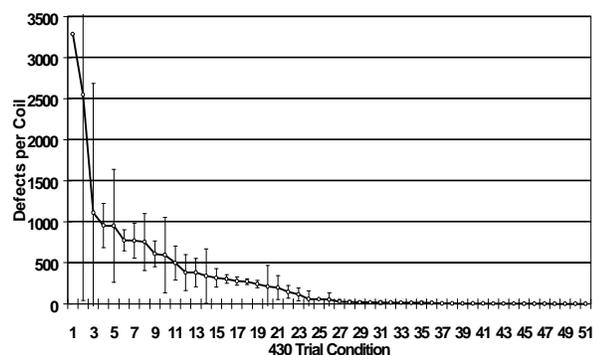
Fig. 22. Reduction in short line defects on 430 stainless at Mansfield by trial condition.
