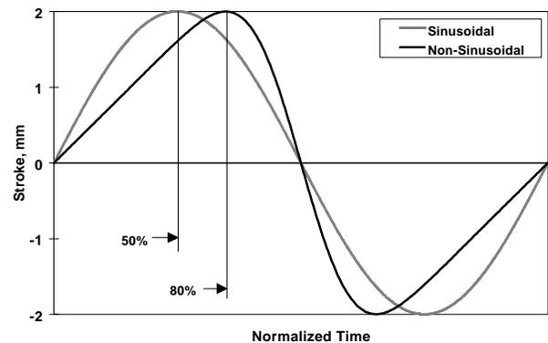
Fig. 5. Range of non-sinusoidal oscillation capabilities.
