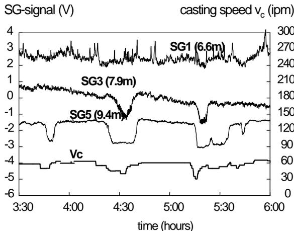
Fig. 19. Typical strain gauge signals.
