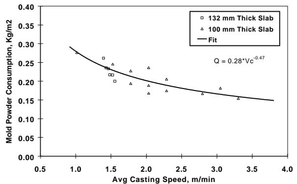
Fig. 9. Mold powder consumption observed on low carbon steels at 4'' and 5.2'' slab thickness with inverse frequency oscillation.
