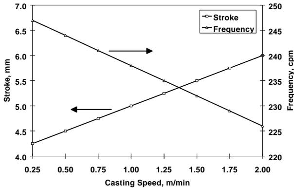
Fig. 6. Typical inverse frequency oscillation practice.
