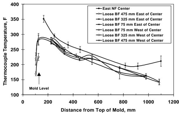
Fig. 12. Typical steady state temperature distribution on the loose broadface for 409 stainless cast at 70 ipm.
