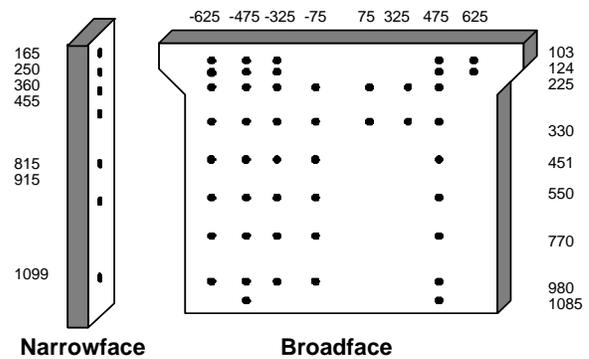
Fig. 10. Thermocouple layout employed on instrumented mold relative to mold top center position, in mm.
