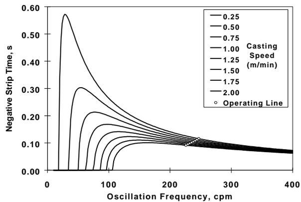
Fig. 7. Mold oscillation operating line with inverse frequency control.
