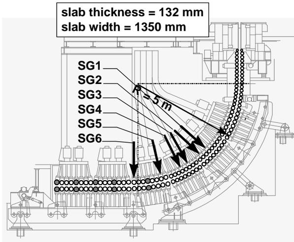
Fig. 18. Location of strain gauges in caster.
