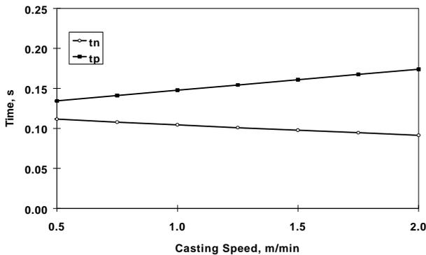
Fig. 8. Typical negative and positive strip times with inverse frequency oscillation.
