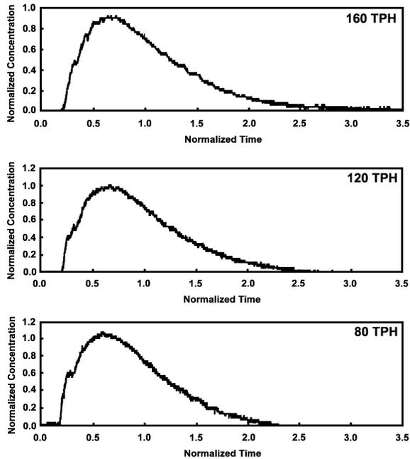
Fig. 3. Tundish residence time distribution plots at 160, 120, and 80 TPH throughputs.
