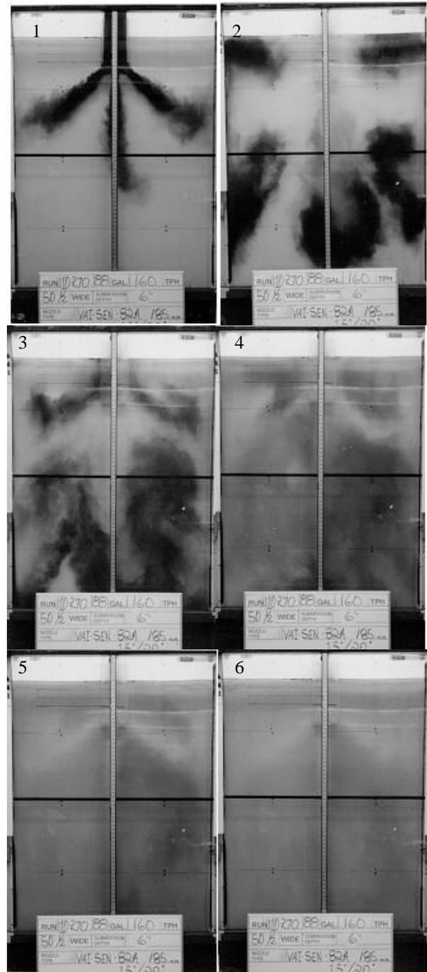
Fig. 4. Visible dye injection sequence in the mold water model at 160 TPH.
