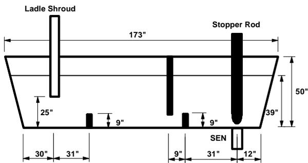
Fig. 1. Tundish flow control configuration for the Mansfield caster.
