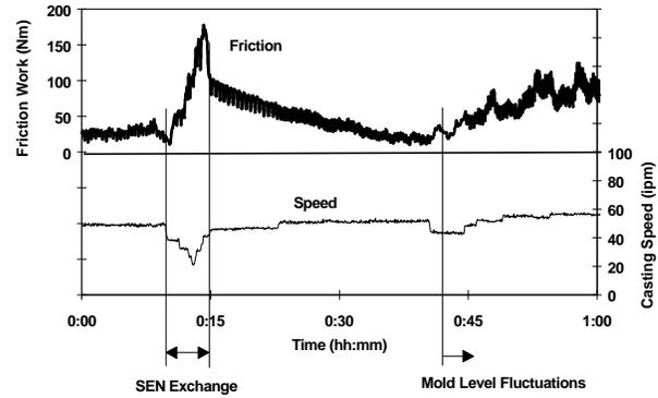
Fig. 17. Typical mold friction trend.
