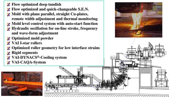
**Fig.2:** Thin slab caster features.
