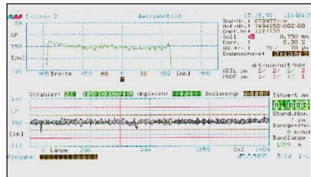
Fig. 11: Cold rolled coil thickness chart.
