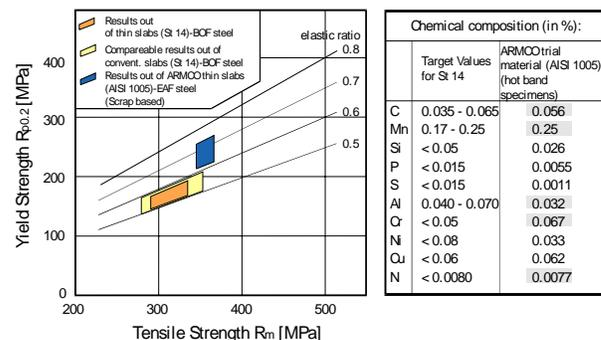
**Fig. 13:** Comparison of mechanical properties of different low carbon steels.
