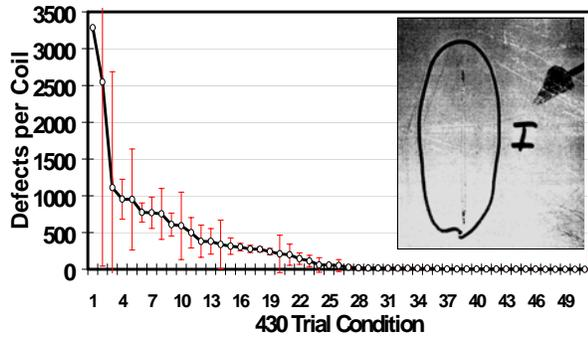
**Fig. 22:** Progress in Reducing Short Line Defects on 430 Stainless at Mansfield.
