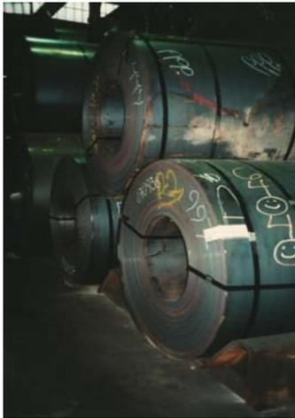
**Fig. 5:** ARMCO coils for cold rolling and deep drawing trials next to the pickling line at VOEST-ALPINE Stahl works, Linz.
