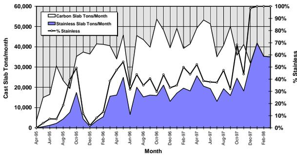
**Fig. 17:** Mansfield Startup Curve and Transition to 100% Stainless Production.
