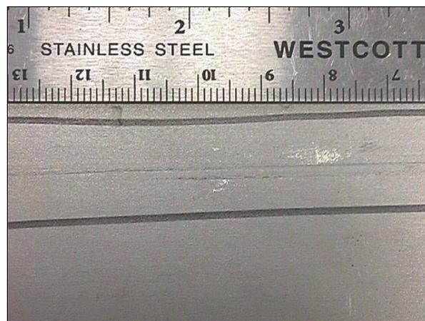
**Fig. 21:** Typical Caster Fold Defect Observed Initially on Annealed and Pickled 430 Hot Band.
