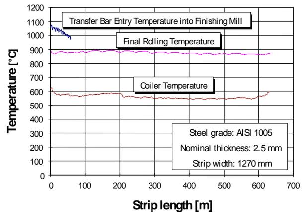
**Fig.7:** Strip temperatures
