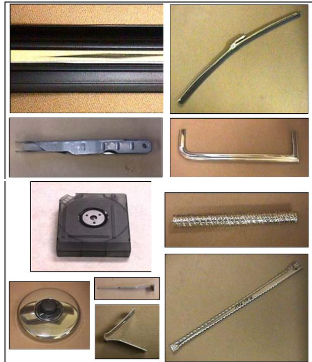
**Fig. 24:** Typical Automotive and Consumer Products Manufactured from Mansfield Produced 430 and 434 Stainless Steel.
