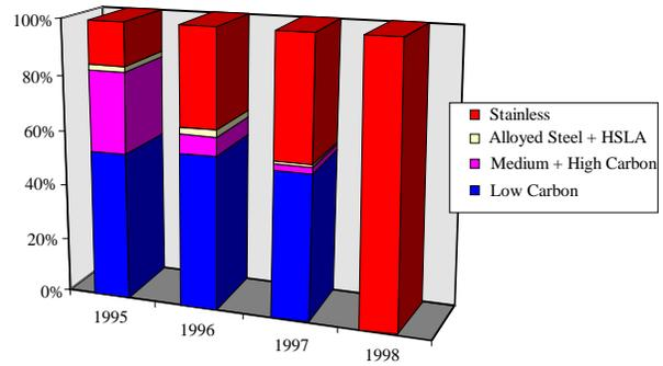
**Fig.3:** Product mix at ARMCO Mansfield since start-up.
