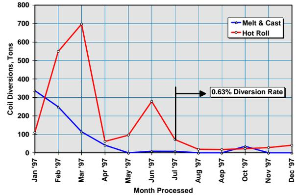
**Fig. 19:** Summary of Cast/Melt and Hot Rolling Related Coil Diversions on 409 Stainless Produced in Mansfield and Processed on #1AP in Zainesville in 1997.
