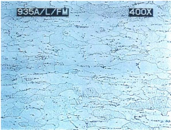
**Fig. 14:** Microstructure of ARMCO cold rolled coil.
