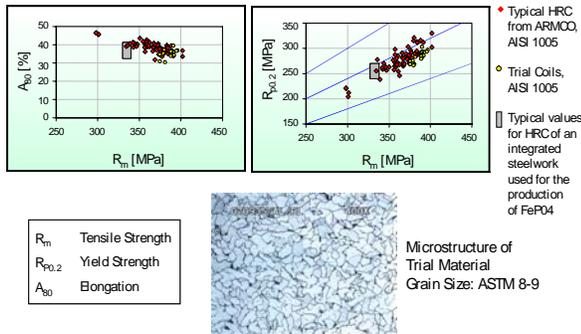
Fig. 8: Mechanical properties of the hot rolled coils.
