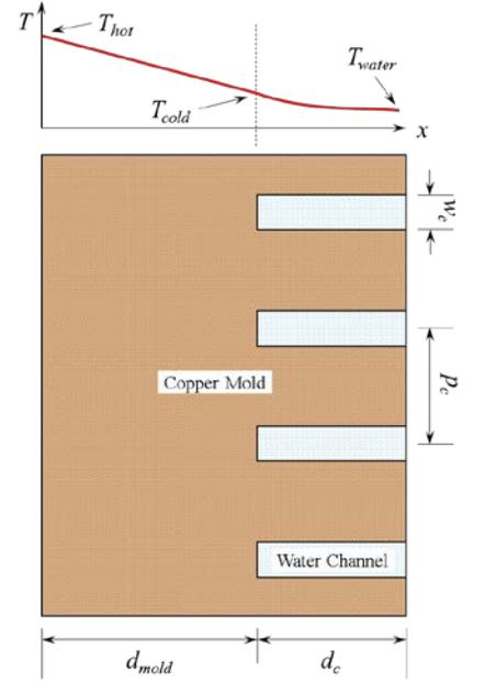
Figure 1. One-Dimensional Mold Model
