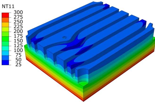
Figure 3. Mold Temperatures (°C) in Mold Calibration Domain from 3D Model (Case 1)
