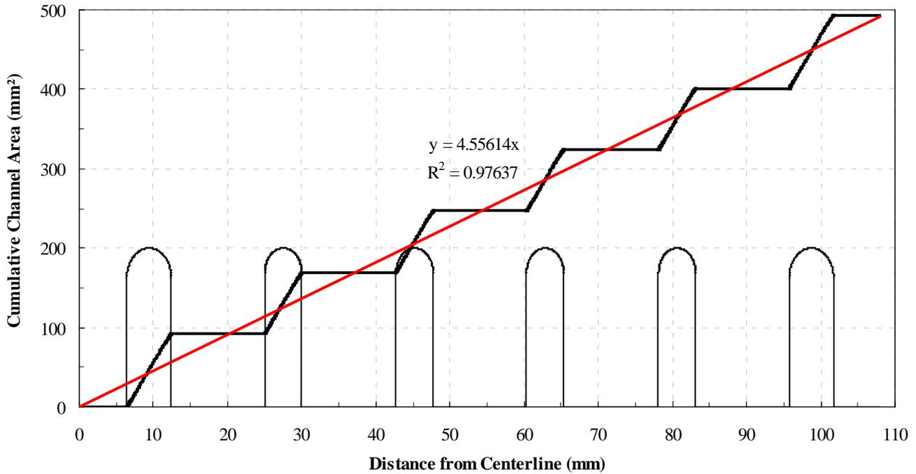
Figure 6. Determination of the One-Dimensional Channel Pitch
