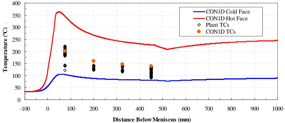
Figure 7. Calibrated CON1D Matches Plant Thermocouple Measurements
