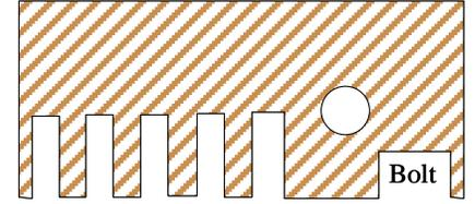
Figure 2. Simulated Channel Pitch Should Match Cumulative Channel Area
