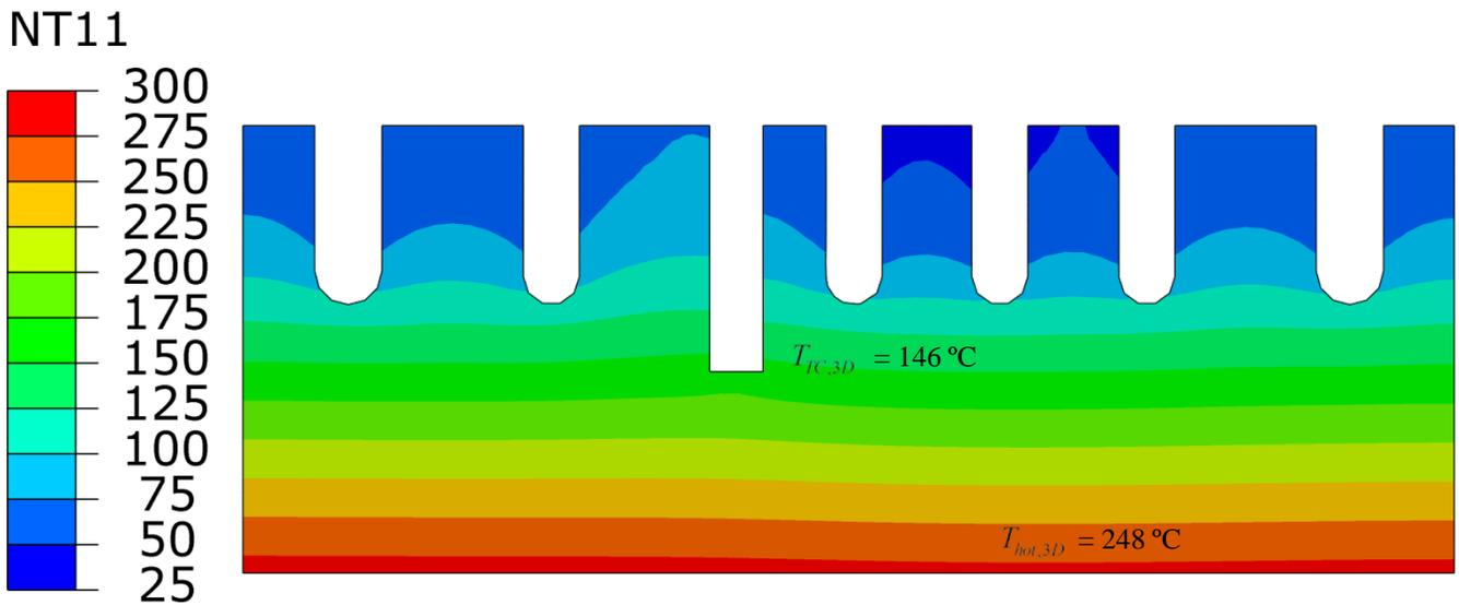
Figure 5. Mold Temperatures (°C) from 3D Model Near Thermocouple (Case 1)
