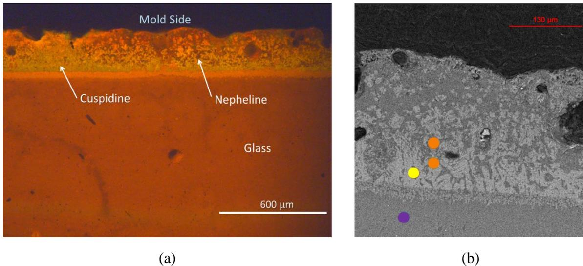
**Figure 7:** CL image (a) and SEM image (b) of the crystal growth along the mold wall. In (b) orange is nepheline, yellow is cuspidine, and purple indicates the bulk glassy region.
