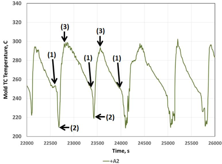
**Figure 5:** Proposed origin of saw tooth temperature fluctuations: (1) fracture of flux crystalline film, (1→2) withdraw of flux crystalline film, (2) air gap, (2→3) inflow of glass, (3) complete glass infiltration, (3→1) aging and crystallization of glass.
