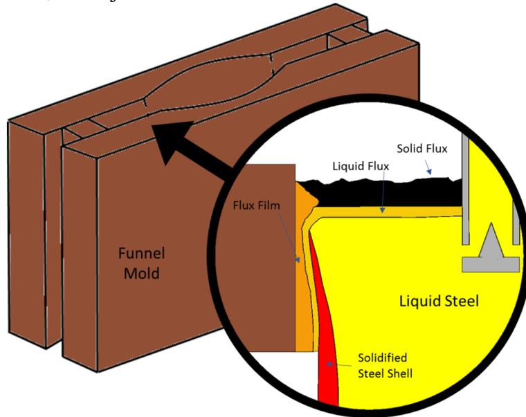
**Figure 1:** Schematic of the funnel mold and the cross section of the mold.
