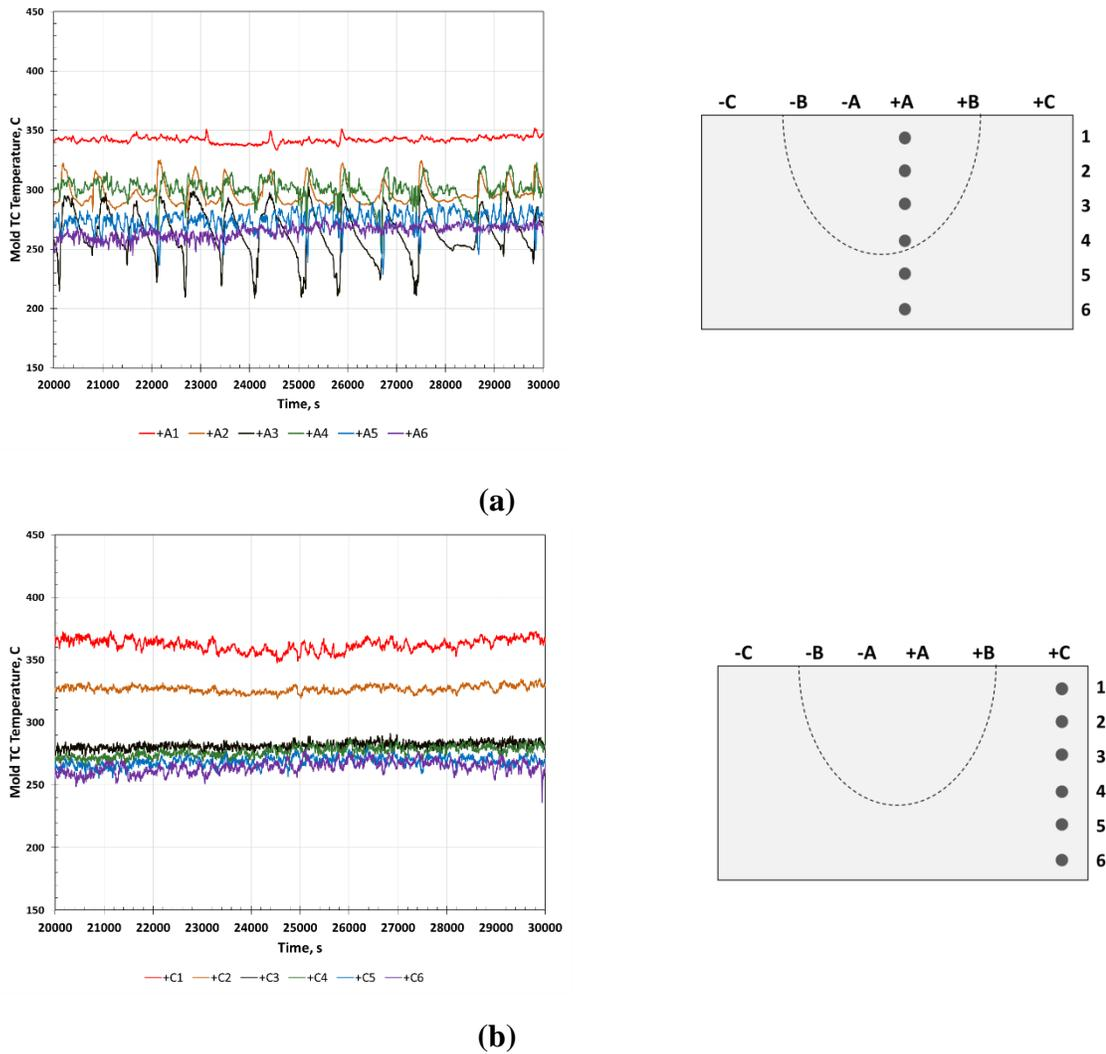
**Figure 3:** Inside the funnel area (a) exhibits saw tooth behavior, where temperature fluctuates on a semi-regular basis with respect to time. Outside the funnel area (b), temperature fluctuations are mild ( $\pm 10^\circ\text{C}$ ). Corresponding diagrams indicate thermocouple locations in the funnel mold.
